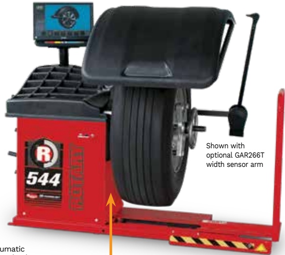
AIR LOCK Pneumatic locking of the wheel.
